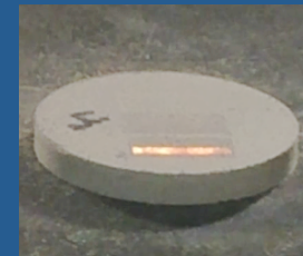
Current Spike During Laser Sintering, Yttria Stabilized Zirconia
